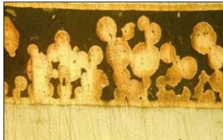
*Fig. 3. Metal-fluoroplastic tape structure (Russia) [1]*
