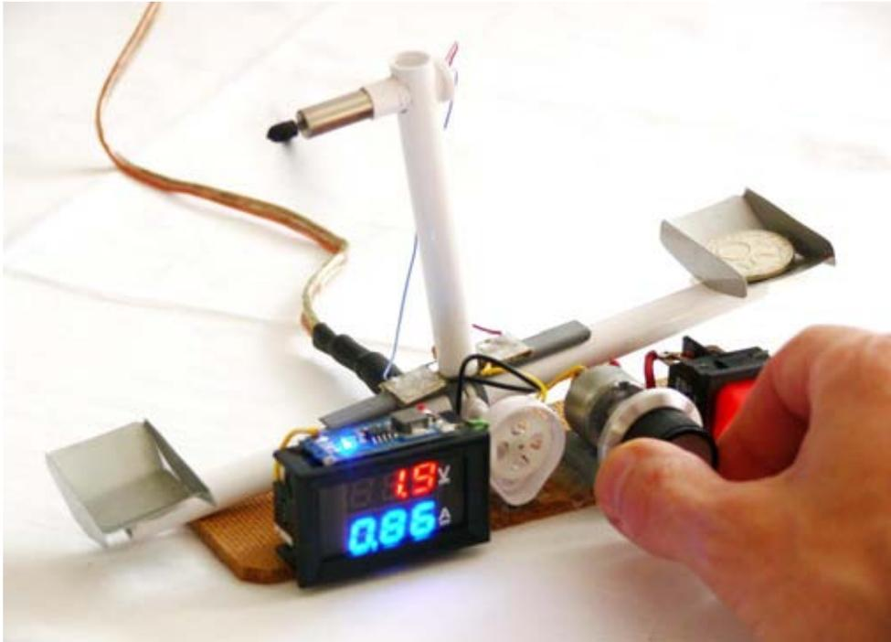
*Fig. 1. Scale for measuring static thrust of micro-motors*
