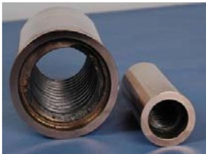
*Fig. 5. Billets of nuts from the material BFG-50M*
